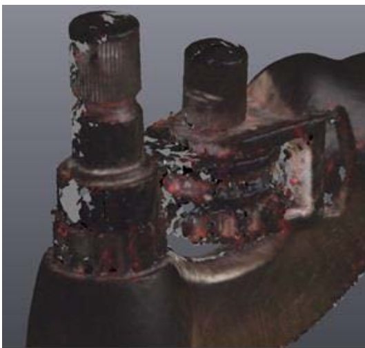
Fig. 11: Detail of the meshed 3D model with 0.2mm accuracy and textures
