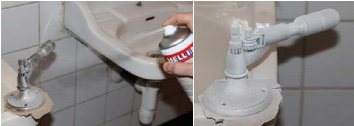
Fig. 13: Spraying of the ring enlarger with titanium oxide (left) to obtain a non-reflective surface (right)
